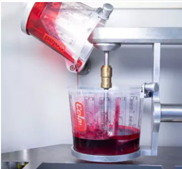
Mixing of PU Resin
