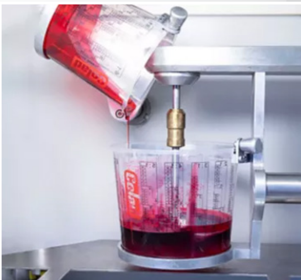
Mixing of PU Resin
